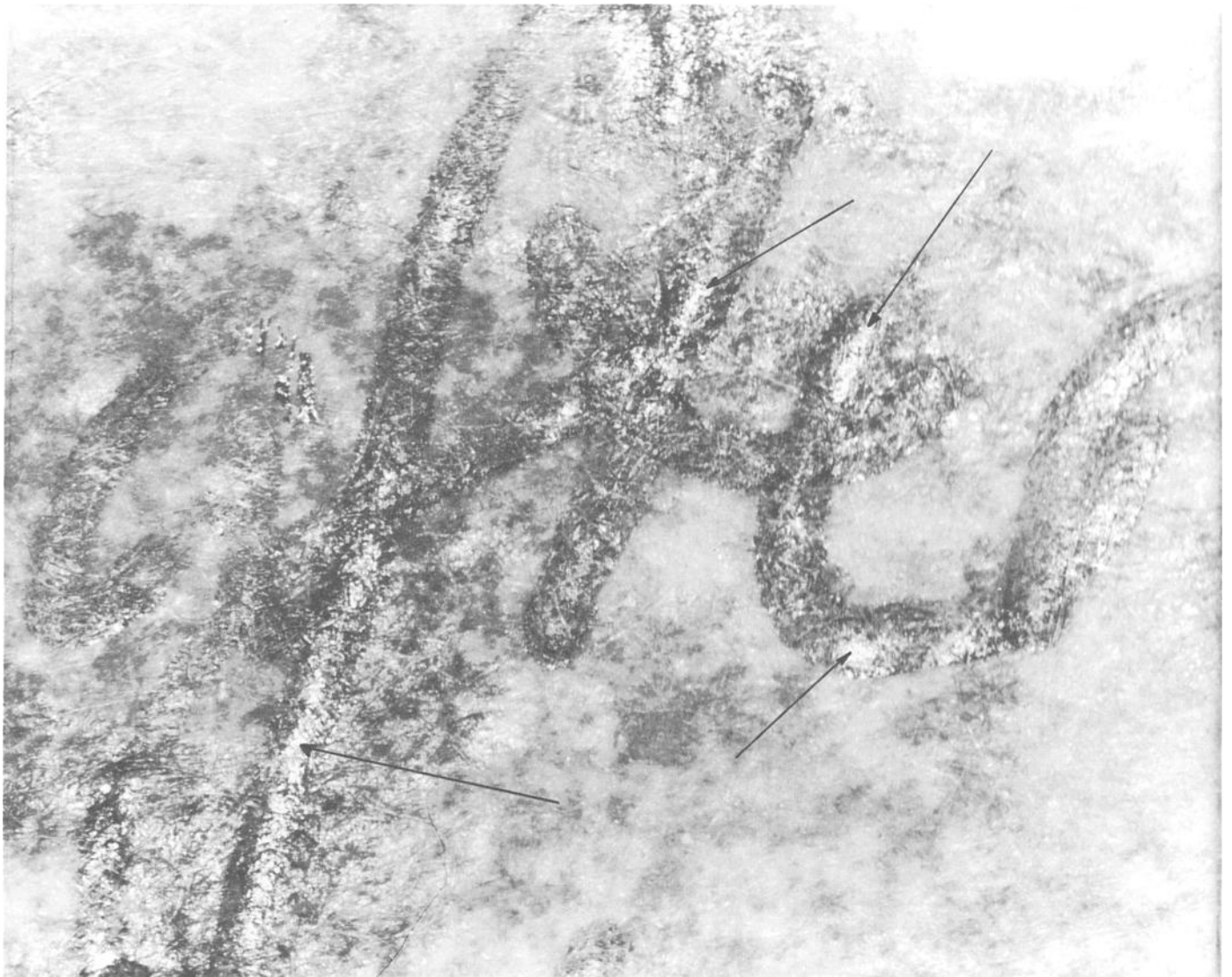
FIG. 2— Specular reflections on ink overlaying blood.
