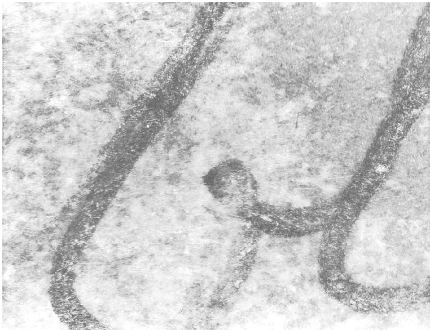
FIG. 3—No specular reflections on blood overlaying ink.
